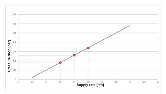
Figure 5.3 Pressure drop at the 3m³/h DHW speed-alternator
