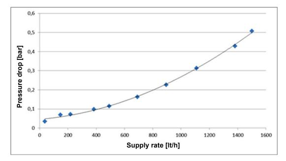
Figure 5.2 Pressure drop at the 1.5m<sup>3</sup>/h DHW speed-alternator
