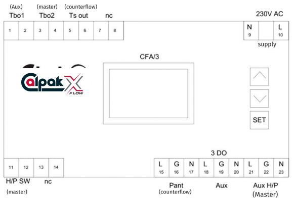
**Figure 11** CFA/3 terminals
