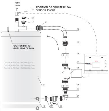
Note: The above drawing applies for models: Calpak X-FLOW 1.5/500 (plus), Calpak X-FLOW 1.5/1000 (plus), Calpak X-FLOW 1.5/2000 (plus)
