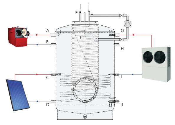
Use B: Heating water with Calpak M4 solar panels, a heat pump and a boiler
