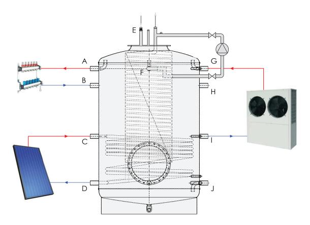
Use C: Underfloor heating and hot water heating using Calpak M4 solar panels and a heat pump
