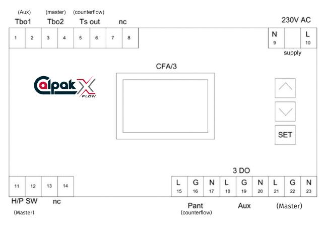
Figure 10 CFA/3 terminals
