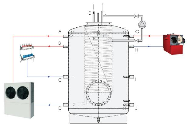
**Use A:** Underfloor heating and hot water heating using a heat pump and a boiler (if the boiler is the main source of energy, then connect it at the positions A and D)
