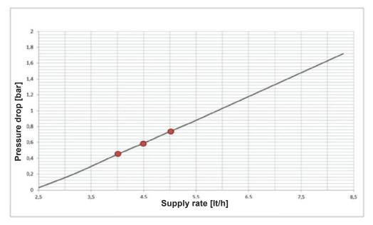
Figure 5.4 Pressure drop at the 4.5m<sup>3</sup>/h DHW speed-alternator
