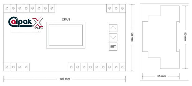
Figure 9 Control unit dimensions
